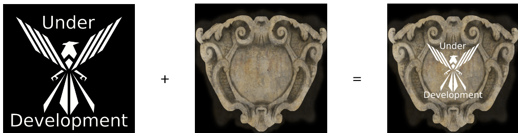
Figure 43: One example of a plugin that can be added to the Blender glTF exporter interface is a watermarking tool that can mark all textures belonging to assets that are still under development.
