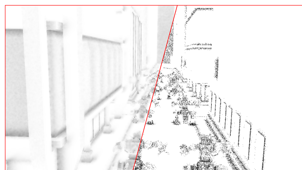
Figure 5: Alternative renderers supported by this framework, such as SVGF filtered Ambient Occlusion with a single sample ray per-pixel (left) and the currently accumulated history length of the SVGF filter (right), the latter of which is a very useful visual milestone while implementing the filter.
