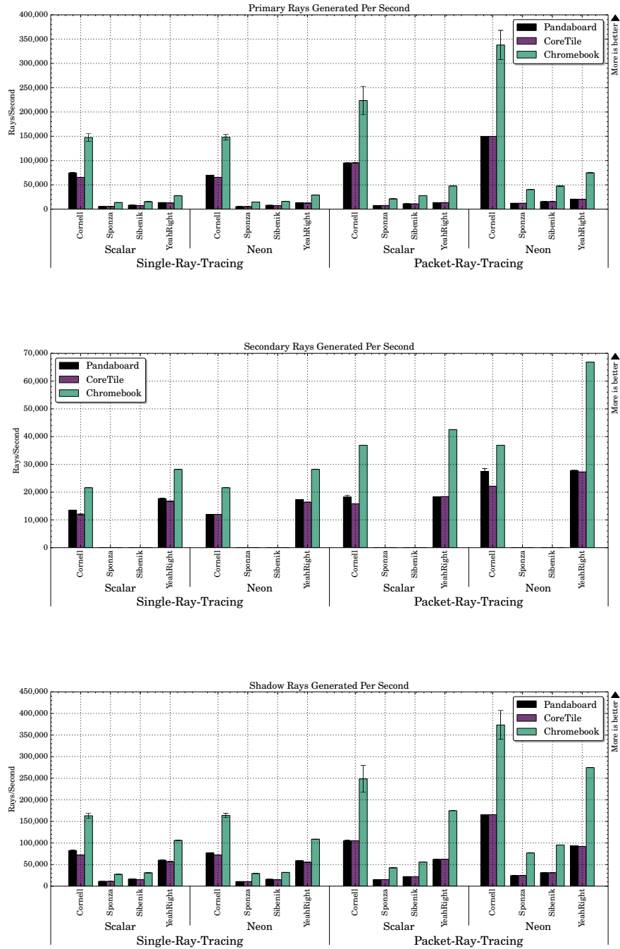
Figure C.5: The computed number of primary, secondary, and shadow rays generated per second during runtime. Note that Spzaza and Sibenik do not contain any specular surfaces, and thus no secondary rays are generated in those scenes.
